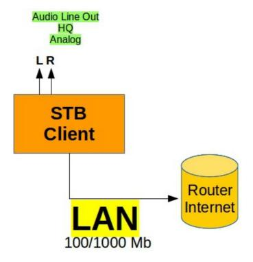
The IP Address is configured by the typical DHCP from the LAN router.
