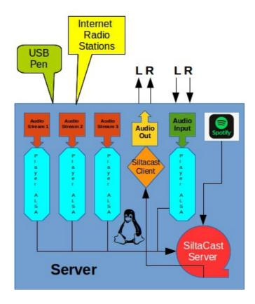
On the server there is a analog output stereo line that allow to perfomance as a normal client.
